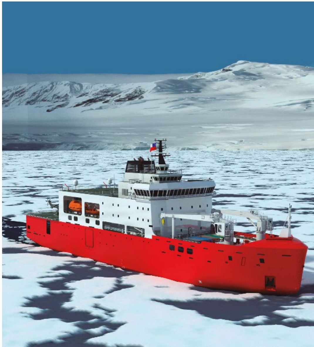
The Chilean Navy's new icebreaker under construction by ASMAR Shipbuilding and Ship Repair Company is based on the Vard 9 203 platform, which is designed to Lloyd's Register PC 5 polar-class notation.
